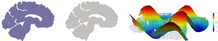
Figure: Triangular mesh of brain section made of 42891 triangles (left), agglomerated polygonal mesh made of 534 polygons (center), and computed PolyDG solution on the polygonal grid with \ell = 1 (right).
