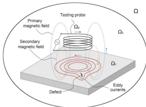
Figure: Sketch of a prototypical ECT setting.
