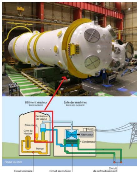
**Figure:** One of the 4 steam generators of an EPR plant (25m high, 510 tons).
