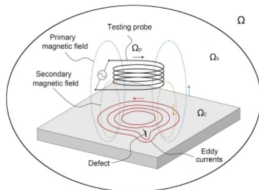
Figure: Sketch of a prototypical ECT setting.
